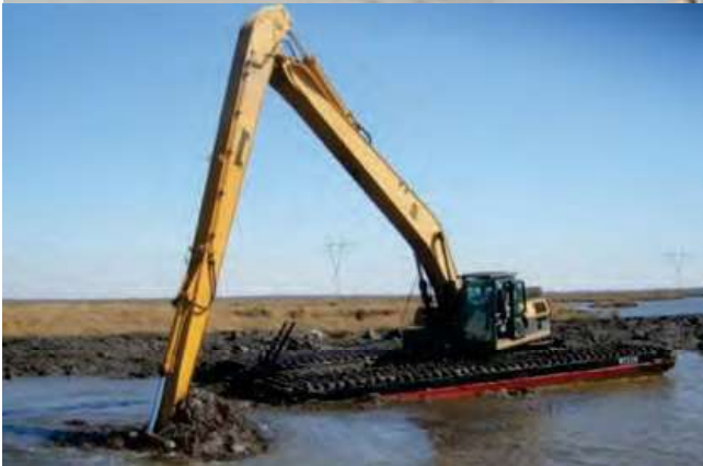
TOP: Cutter suction dredge and floating pipeline. Image courtesy Van Oord. UPPER MIDDLE: Dredge material placement. Image courtesy USACE Mobile District, Building Ship Island. LOWER MIDDLE: Pipeline spread for dredge material placement. BOTTOM: Low ground pressure amphibious excavator.
