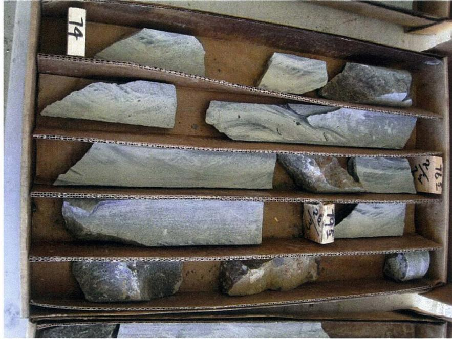
**PHOTOGRAPH 7.** Basalt boulders and cobbles with no fines in DOB08DH-03
