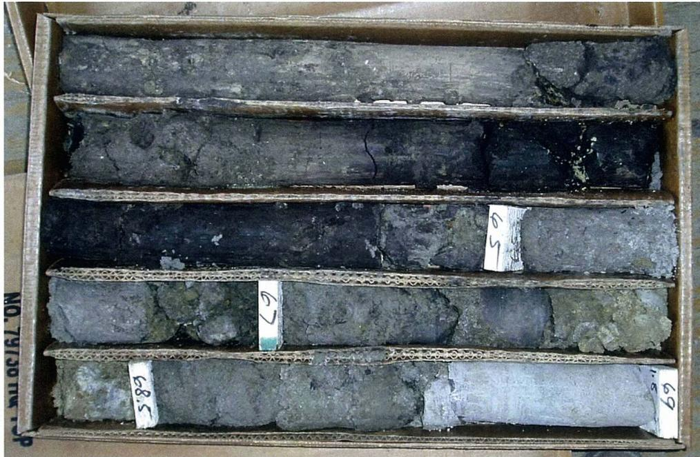
**PHOTOGRAPH 3.** Clay in Lower Tuff unit in DOB05DH-06
