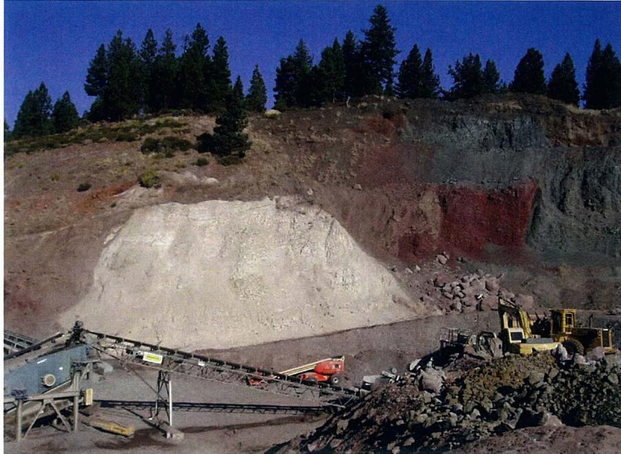
**PHOTOGRAPH 11.** 45-ft high exposure of ash in northwest wall of East Pit
