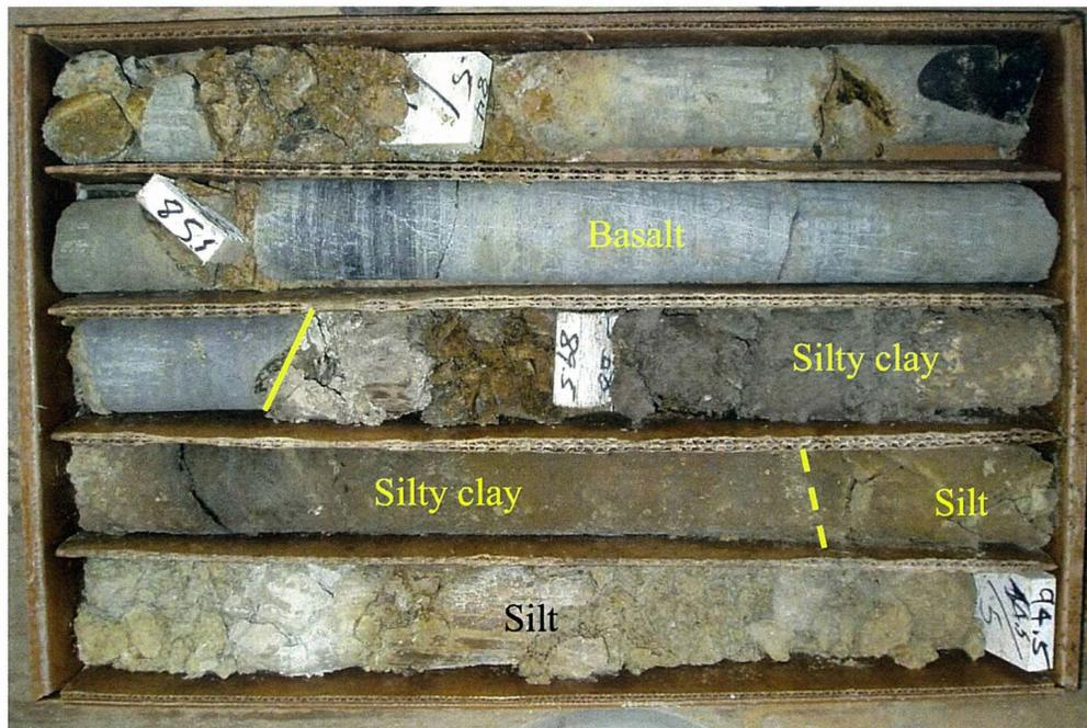
**PHOTOGRAPH 4.** Clay and silt in lower tuff in DOB05DH-07
