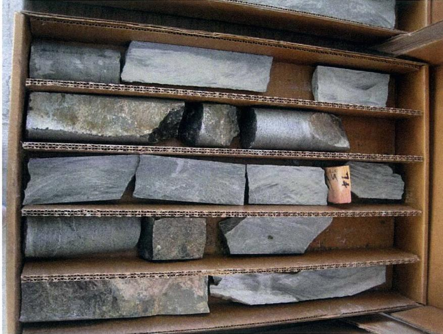
**PHOTOGRAPH 5.** Typical basalt in DOB08DH-02
