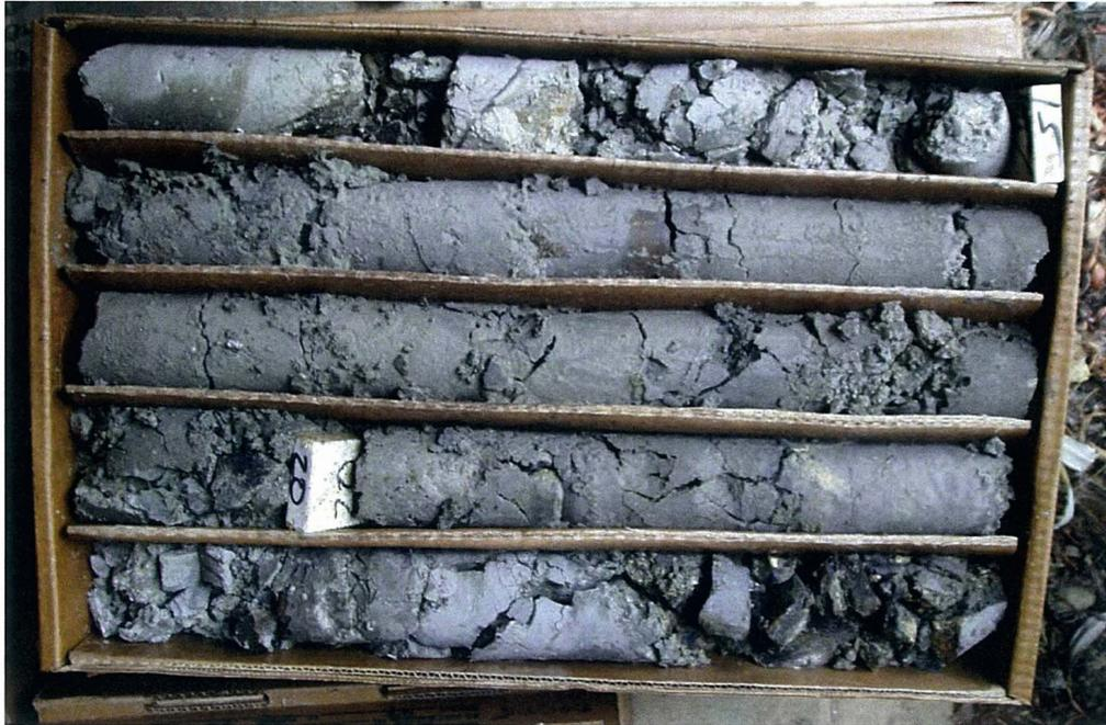
**PHOTOGRAPH 1.** Weak, highly fractured Upper Tuff in DOB05DH-08
