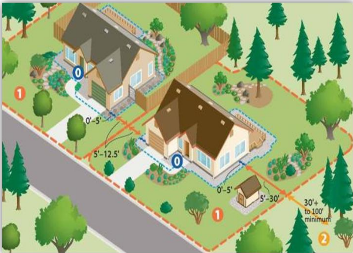
100 ft Defensible Space in a neighborhood.
