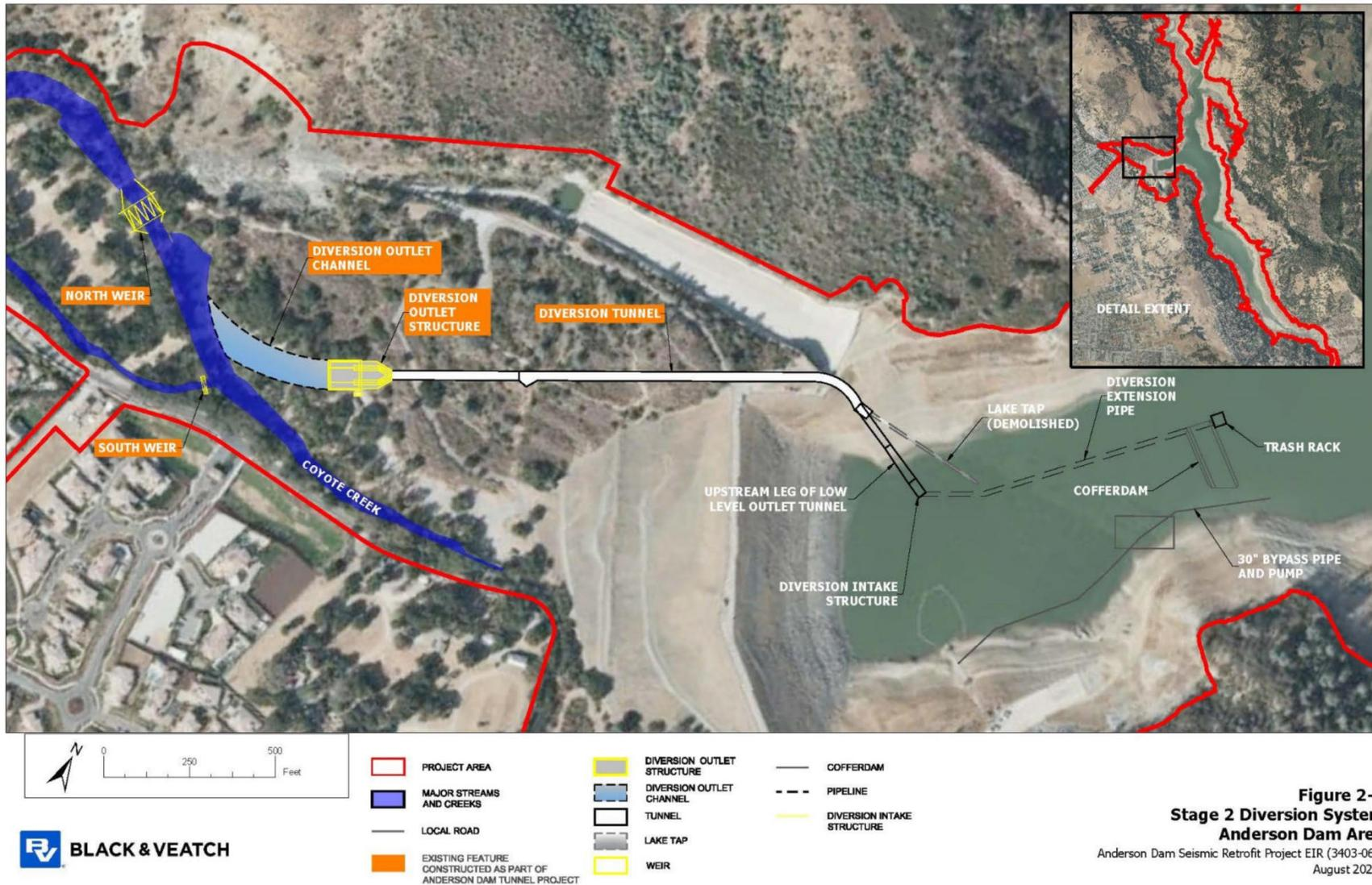
1 **Figure 2-7. High-Level Outlet Works System**
