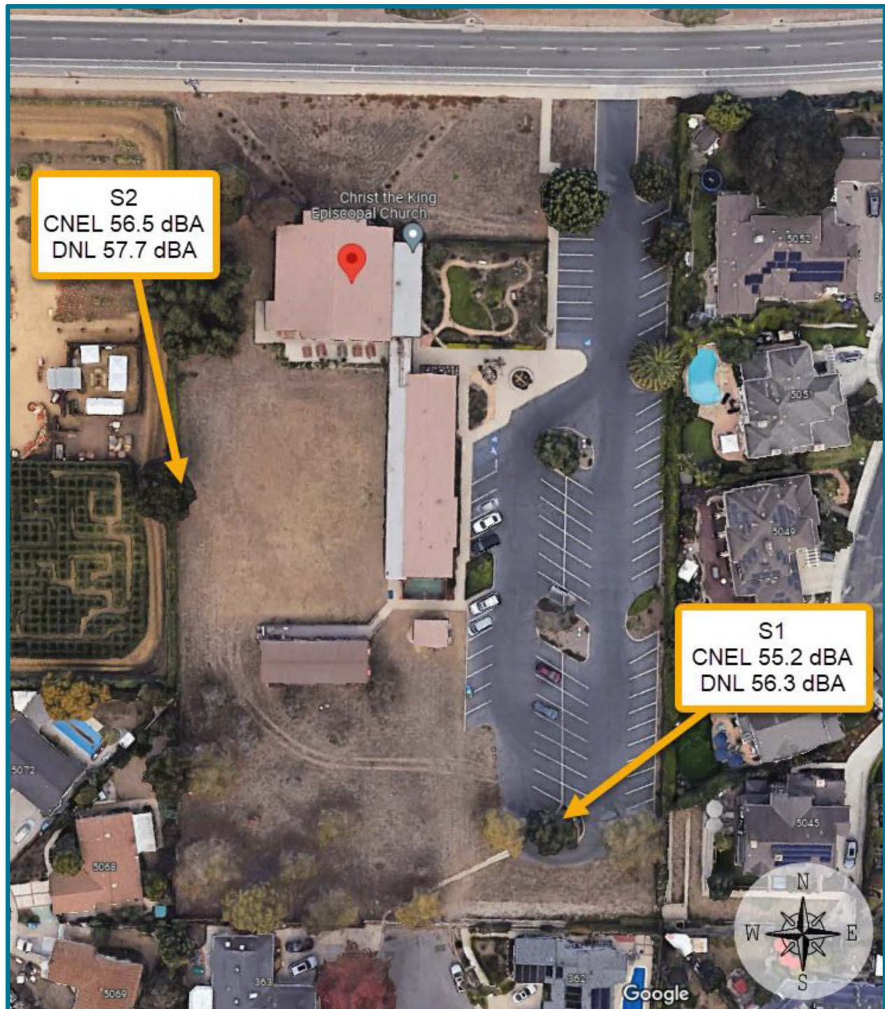
Figure 4: Existing Sound Level Measurement Locations
