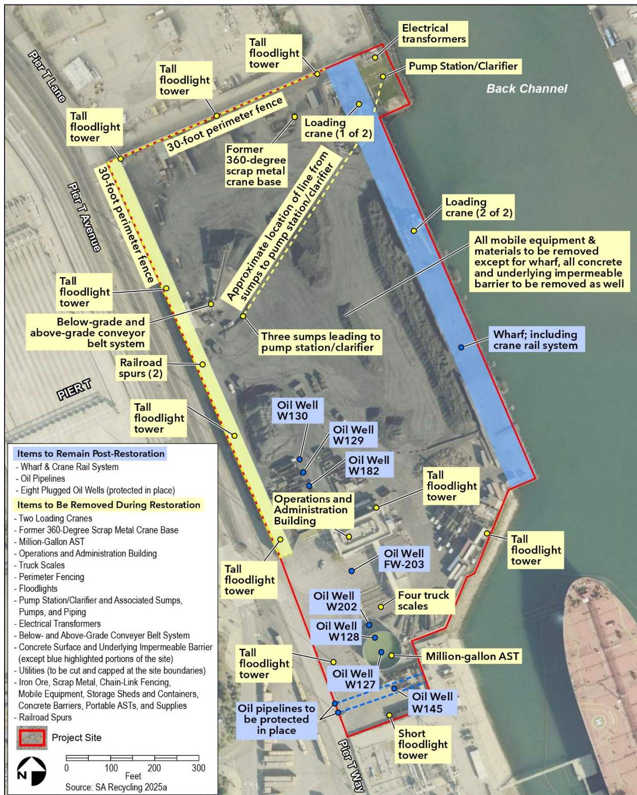
Figure 2-5. Pre-Restoration Site Plan
