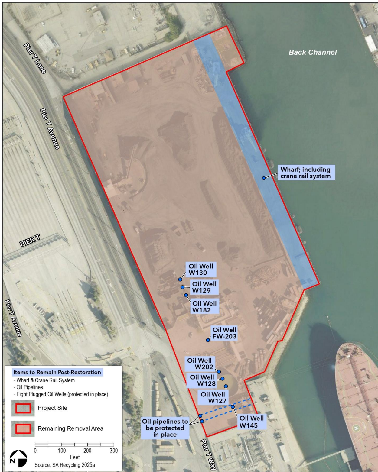
Figure 2-6. Post-Restoration Site Plan
