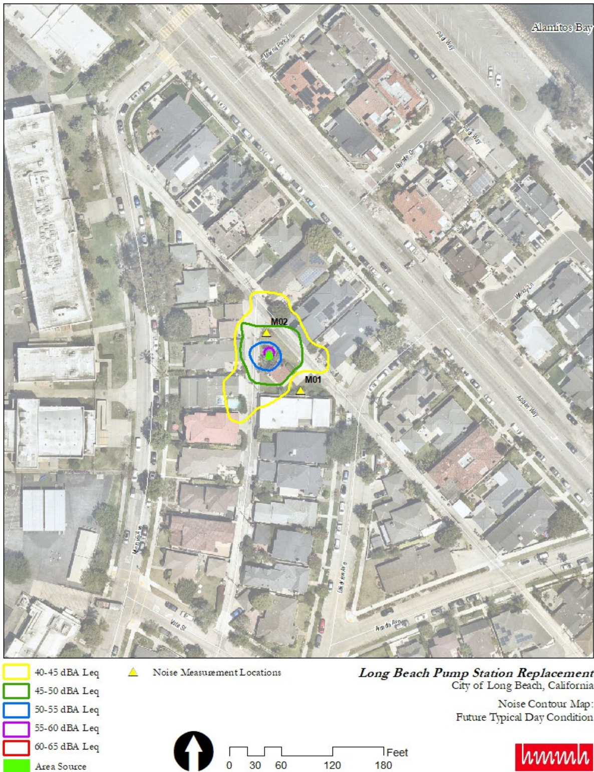
Figure 6. Future Typical Daytime S-7 Operation
