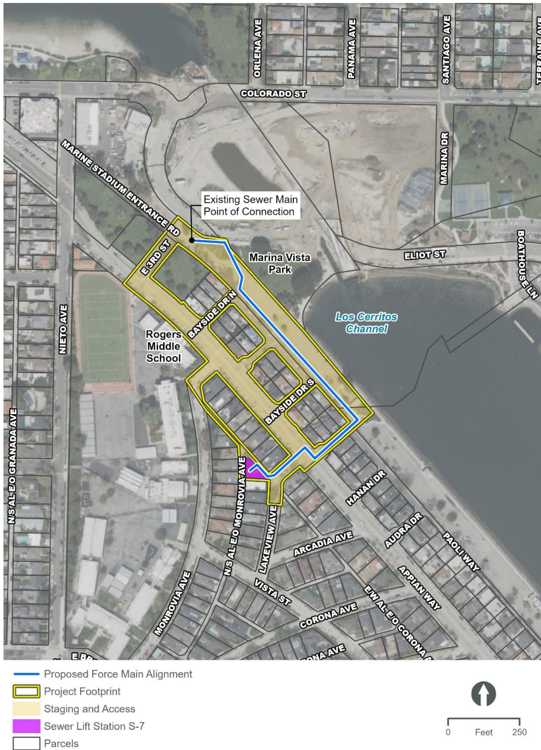
Figure 1: Aerial imagery showing part of Belmont Park neighborhood covering Sewer Lift Station S-7, proposed force main alignment, and the Project footprint. The Sewer Lift Station S-7 property is referred to as the “Project Site”.
