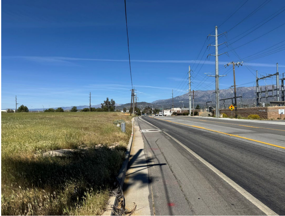
Exhibit 1.9. Southeast driveway looking left (north) – 250-ft sight distance achieved
