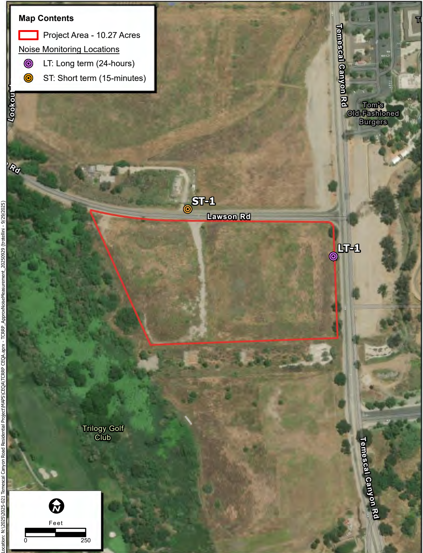
Figure 3. Approximate Noise Monitoring Locations
