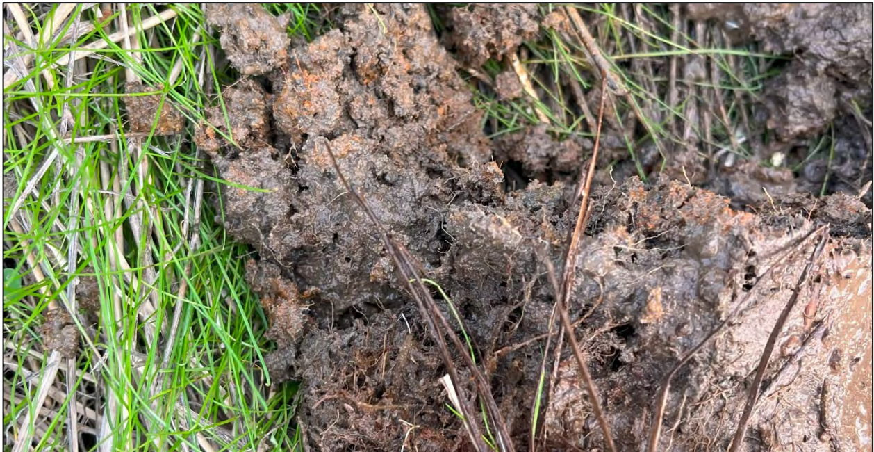
Soils from sample point A-01 (ditch wetland) with substantial amount redoximorphic features (oxidized iron) and saturation to the surface.
