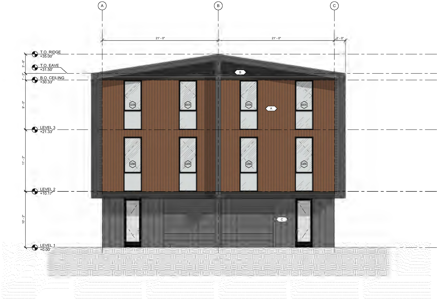
1 TYPE B - FRONT ELEVATION 1/4" = 1'-0"
