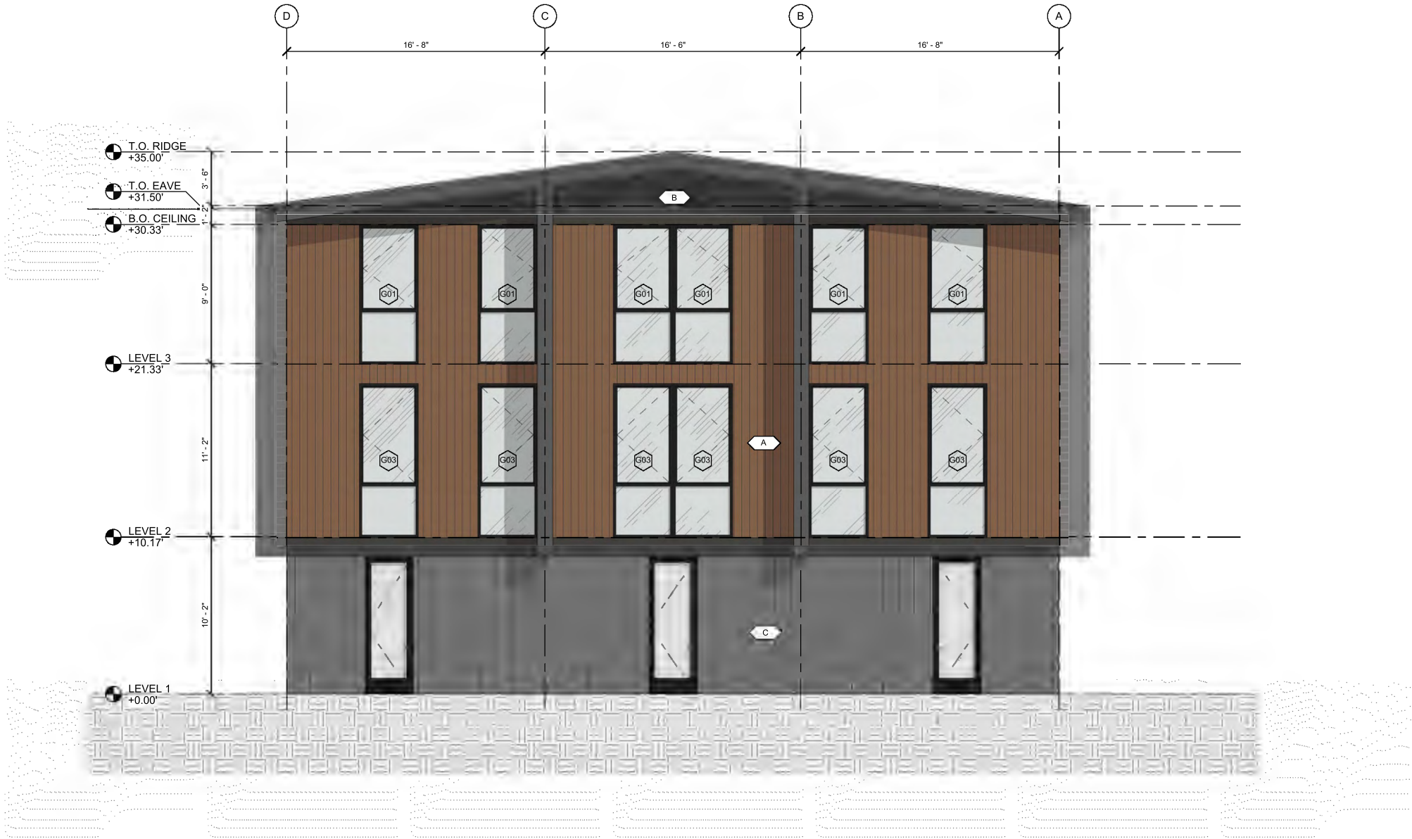
1 TYPE A - REAR ELEVATION 1/4" = 1'-0"
