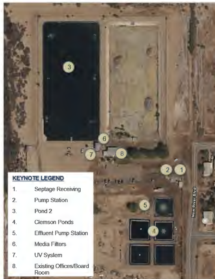
Figure 1-3: Existing Site Layout
