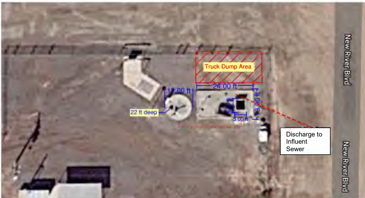
Figure 5-1 Existing Septage Receiving System Layout
