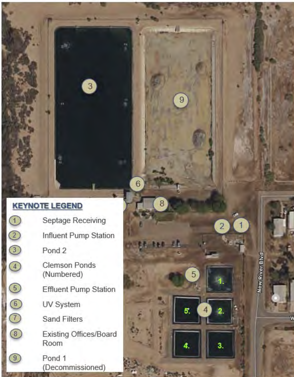
Figure 2-1: Existing Site Layout
