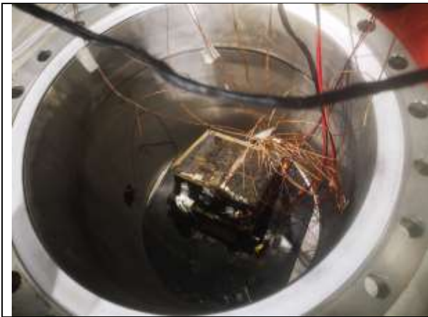
Figure 25: Sample 5 instrumented and inside gas test chamber
