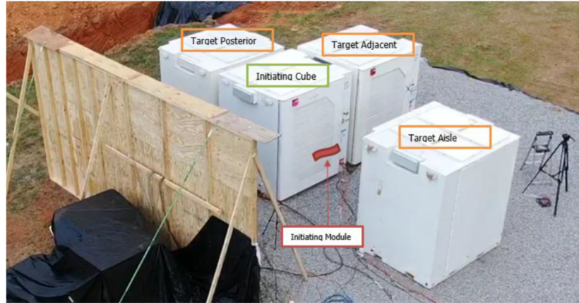
Figure 4. UL 9540A Unit Level Test Layout
