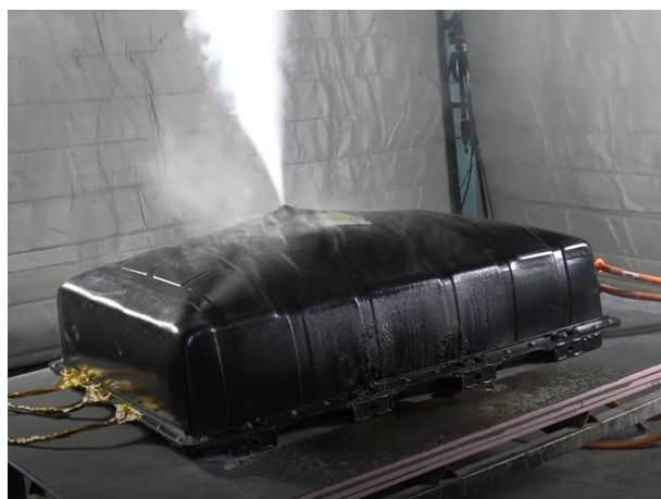
(f) Propagation to Cell 21 (2 nd Thermal Runaway) [01:21:16]
