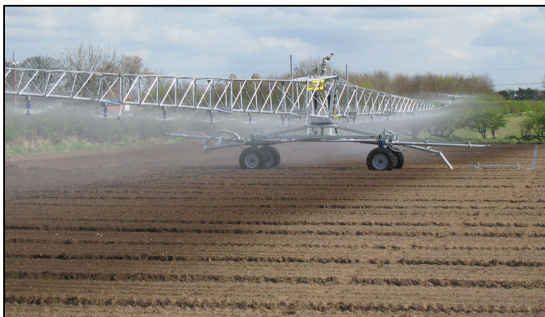
Figure 5. Example of Hose Reel and Irrigation Boom
