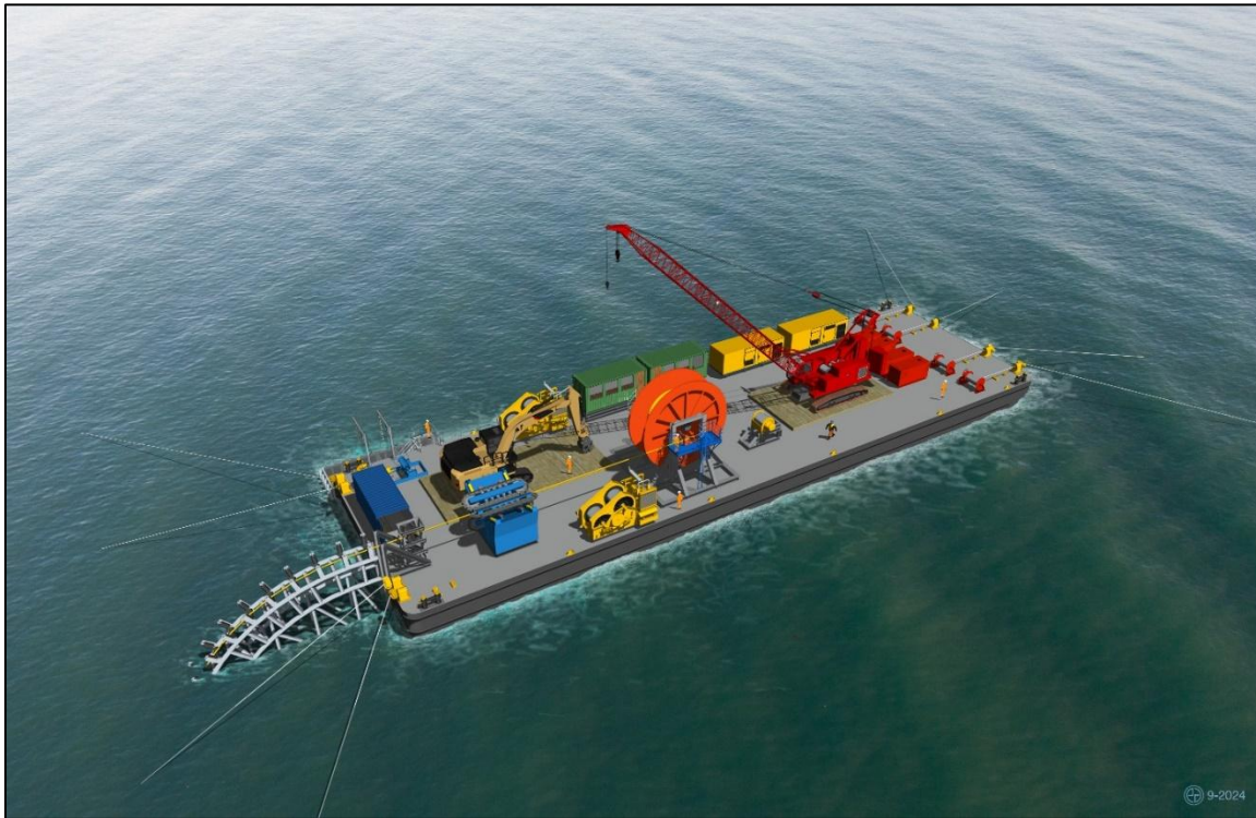
Figure 9. Schematic of Reverse Cable-Lay Barge Support Vessel
