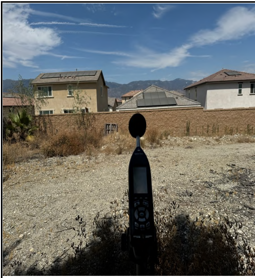
STNM3 looking NE towards back yard wall of residence 2356 Powell Drive, Rialto. Wall is ~50' NE of STNM3 microphone, constructed out of cinder block and is ~6' tall.
