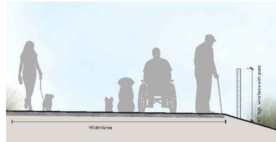
PERIMETER TRAIL AND RESOURCE PROTECTION FENCE CONCEPTUAL SECTION - Not to Scale
