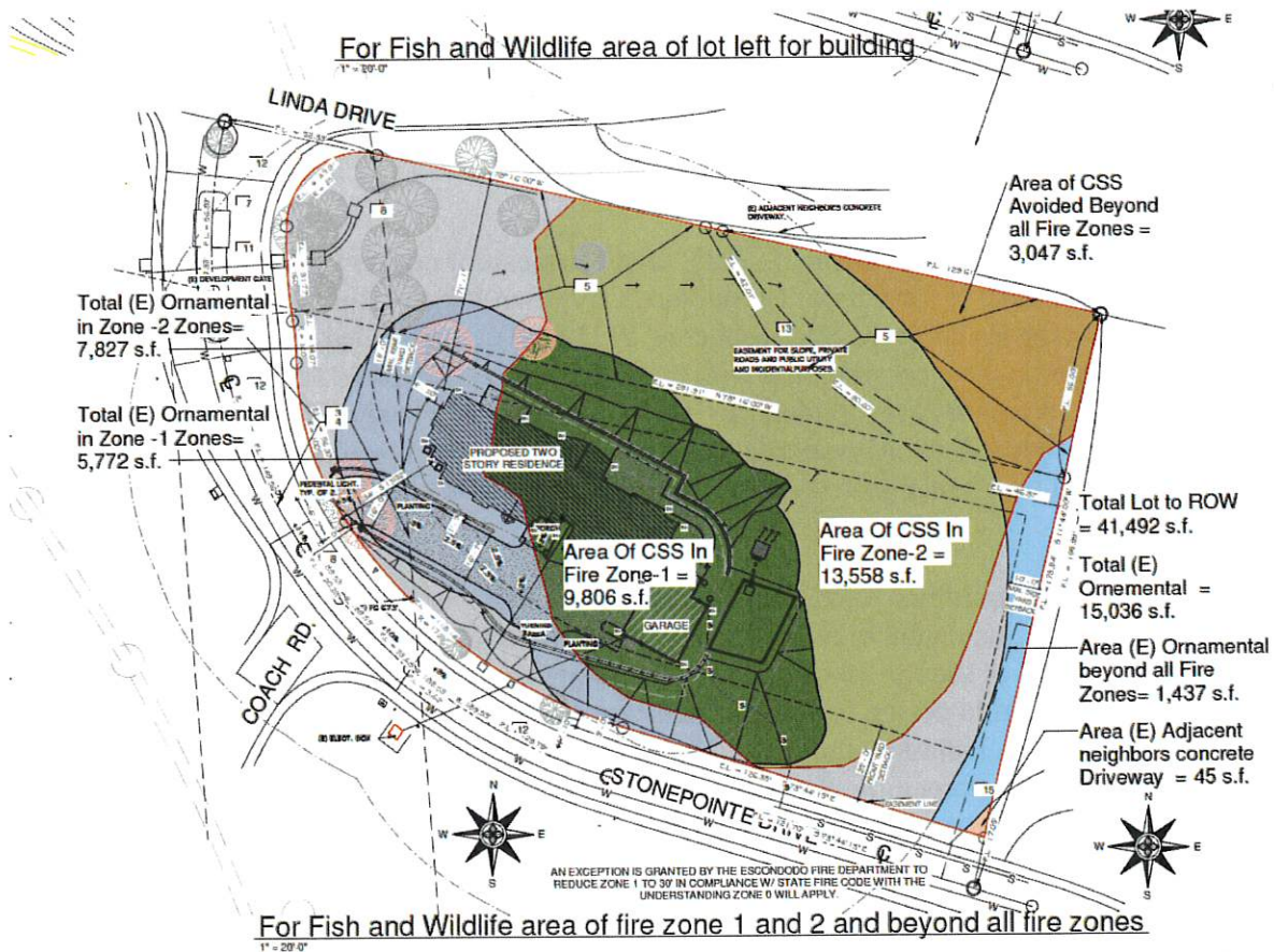
Figure 1. Project Footprint and Fire Zones.
