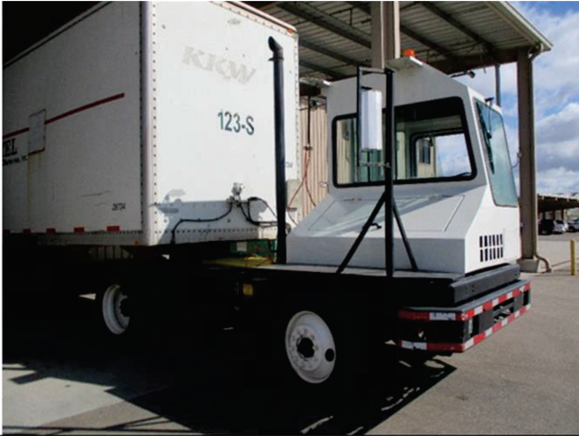
Yard mule (diesel). 1 currently, no additional with expansion
