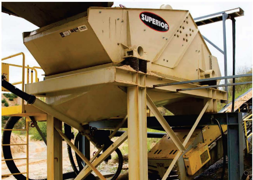
Figure 2-10 Proposed Single-Deck Dewatering System
