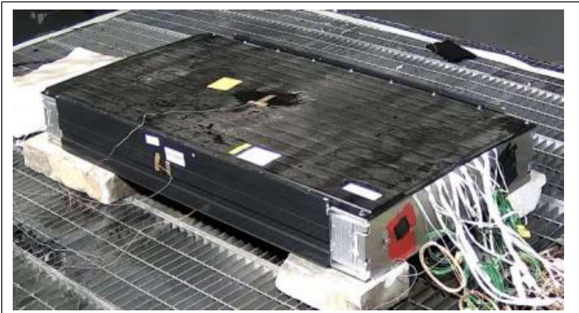
Figure 9: Tray Tested to UL 9540A Module Level Testing
