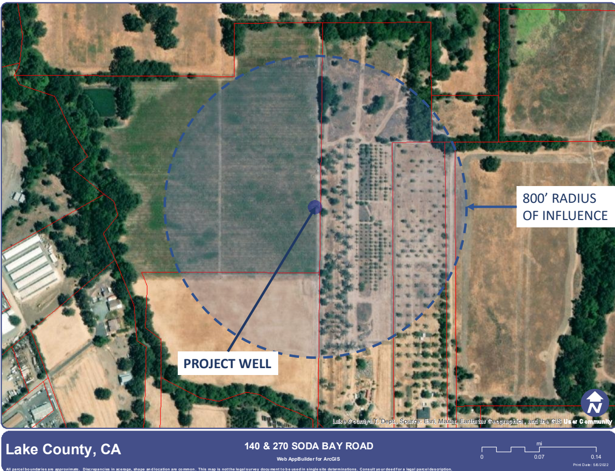
Figure 2 – Zone of Pumping Influence Diagram
