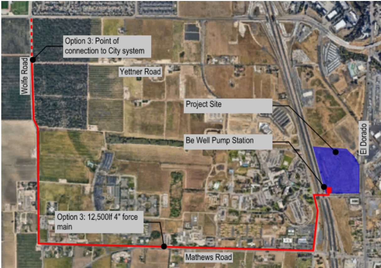
Figure 2: Option 3 Sewer Routing
