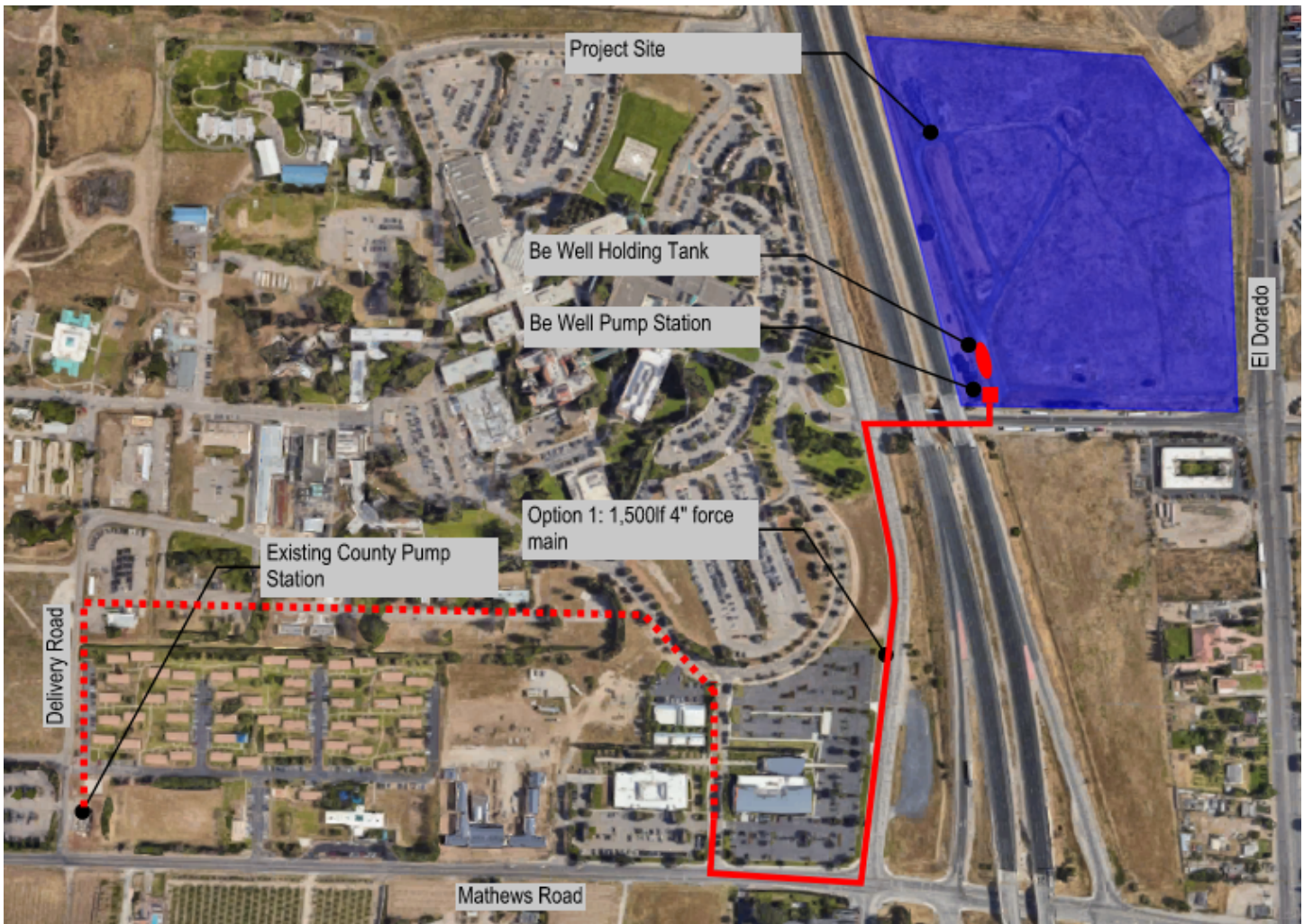
Figure 1: Option 1 Sewer Routing
