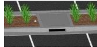
Horizontal Flow Biofiltration System
