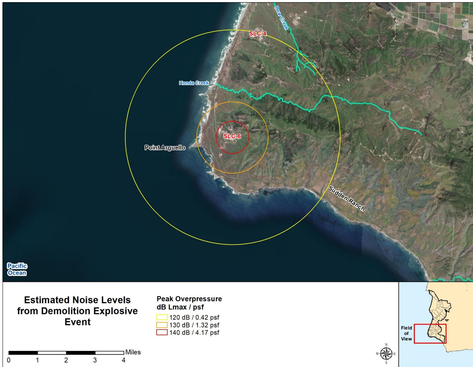
Figure 2.2-3. Estimated impulsive noise levels from explosives used during demolition.
