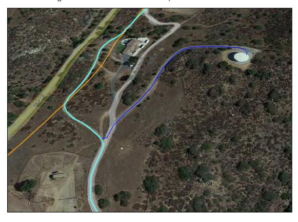
Figure 18: Tank 5 Connection with Proposed Potable Water Line
