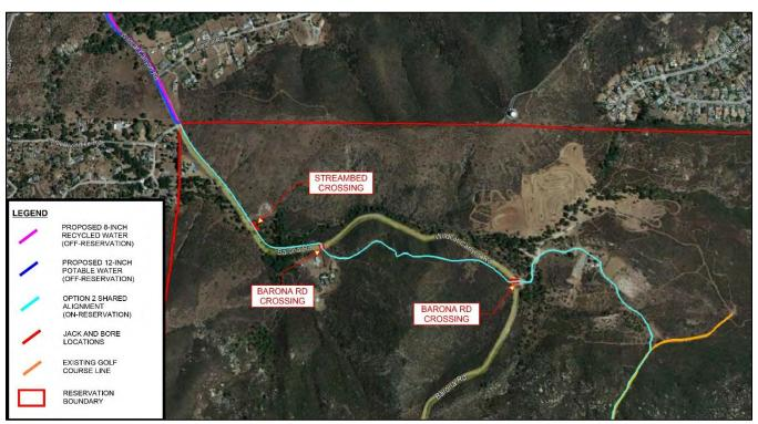
Figure 14: Option 2 On-Reservation Shared Alignment, with Jack and Bore Construction Extents
