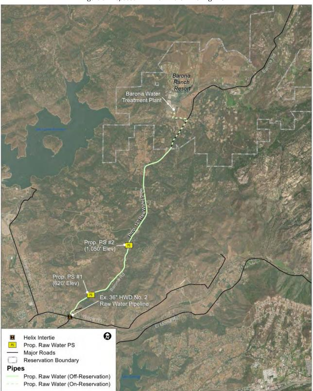
Figure 7: Proposed HWD Raw Water Line Alignment
