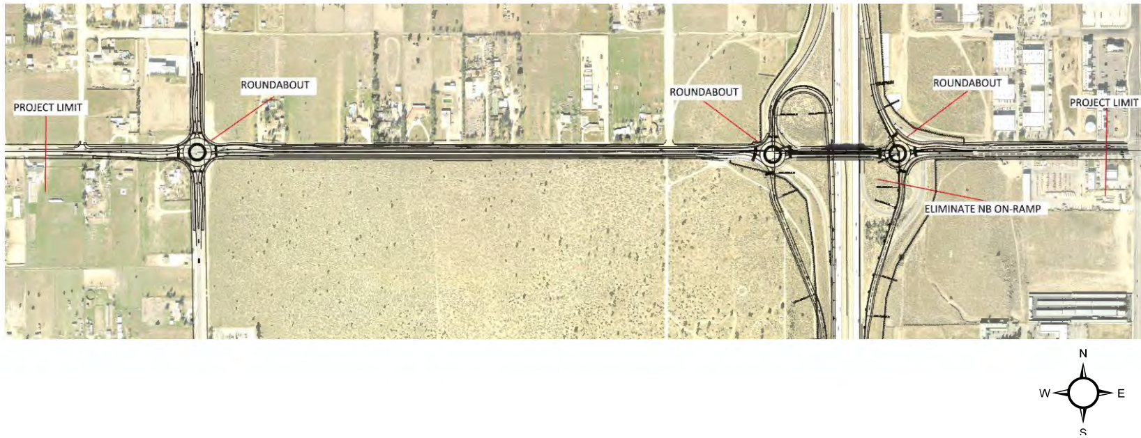
Figure 2-5 Alternative 6 (Interim) Design Elements (Roundabouts at Intersections - One Lane on Avenue M & Elimination of North bound On-Ramp)
