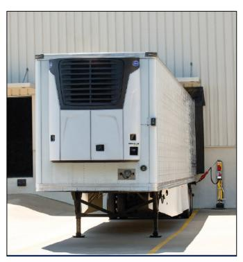
BAC noise level measurement data indicates that diesel TRUs and eTRUs generate average noise levels of approximately 63 dB and 56 dB (respectively) at a reference distance of 100 feet with a direct view of the TRU. As indicated in Figures 6 and 7, positions located behind the trailer are shielded from view of the TRU by the trailer itself and are, therefore, exposed to lower noise levels. Similarly, trailers parked adjacent to each other will provide sideline shielding.
