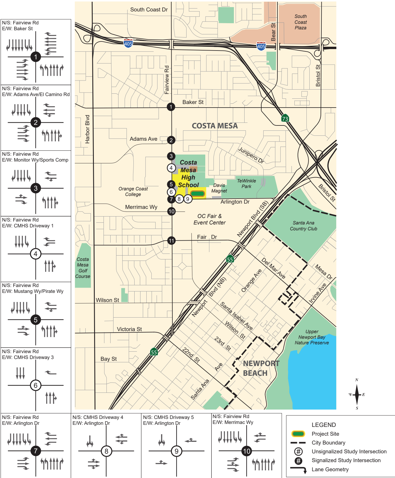
FIGURE 3.1: STUDY INTERSECTION GEOMETRY AND CONTROL
