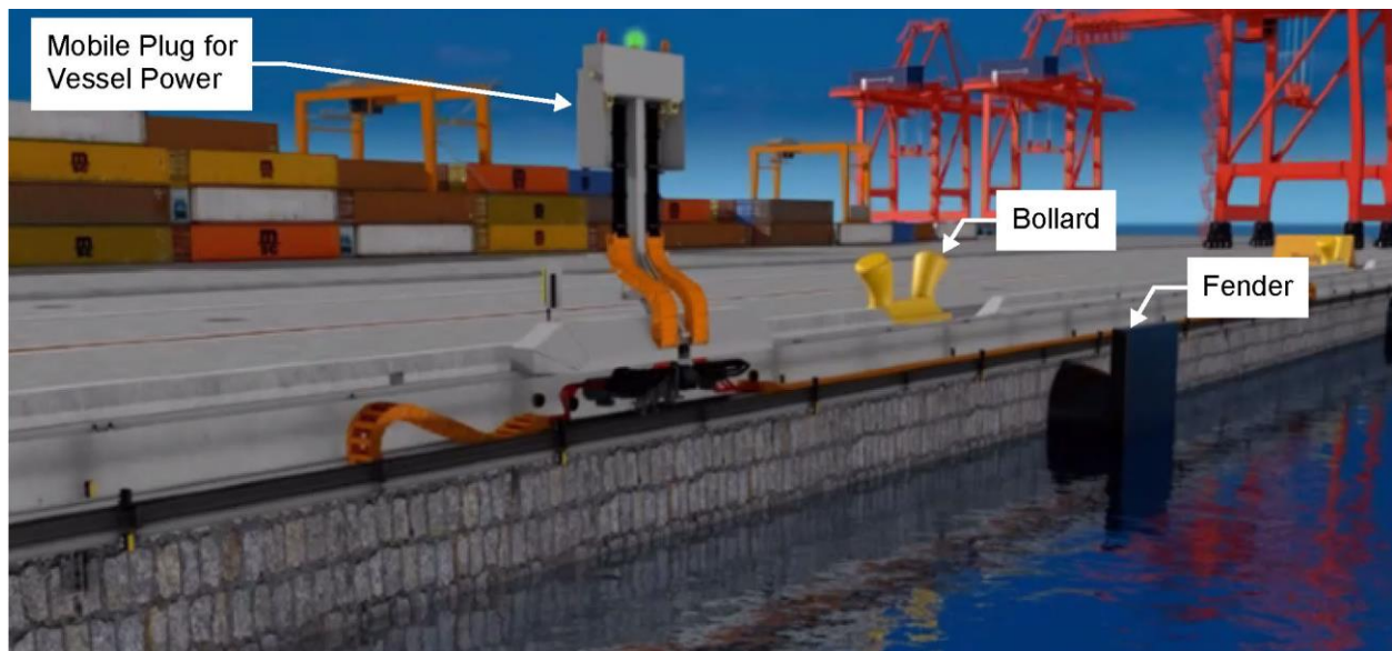
Figure 2-4 Fender, Bollard, and Power Plug-in
