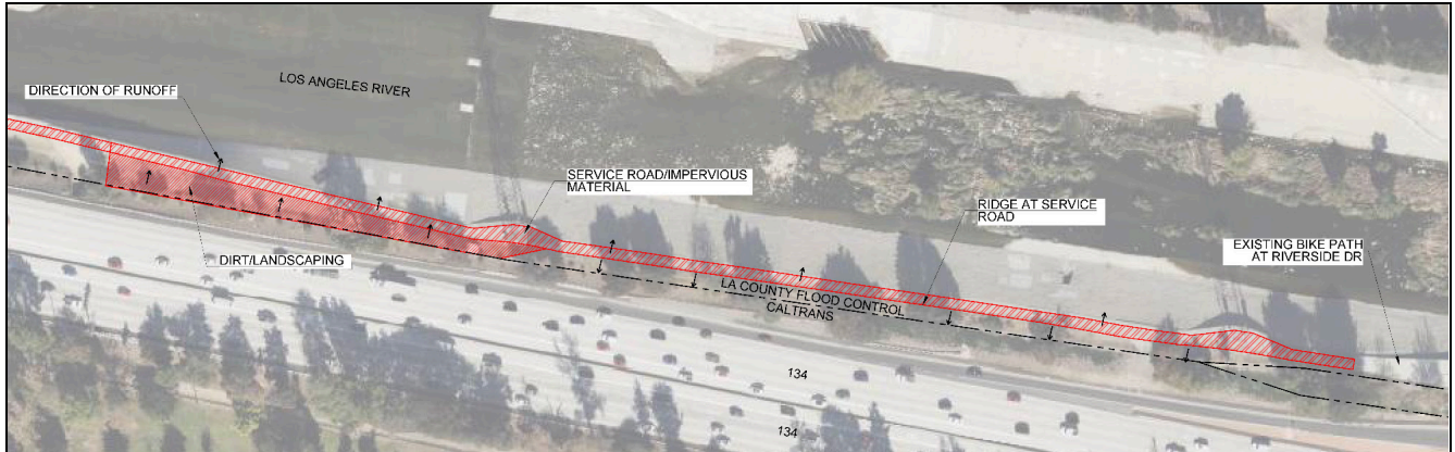
Figure 12: Drainage sub-area A-1 at east end of project site. Run-off flowing across the service road toward the channel
