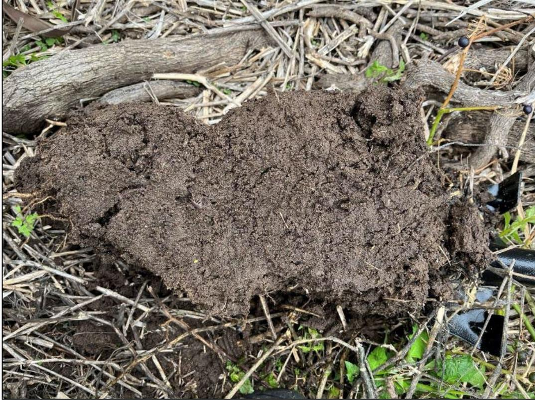
**Figure 4-9.** Hydric soil from culvert 9 with sandy dark surface.
