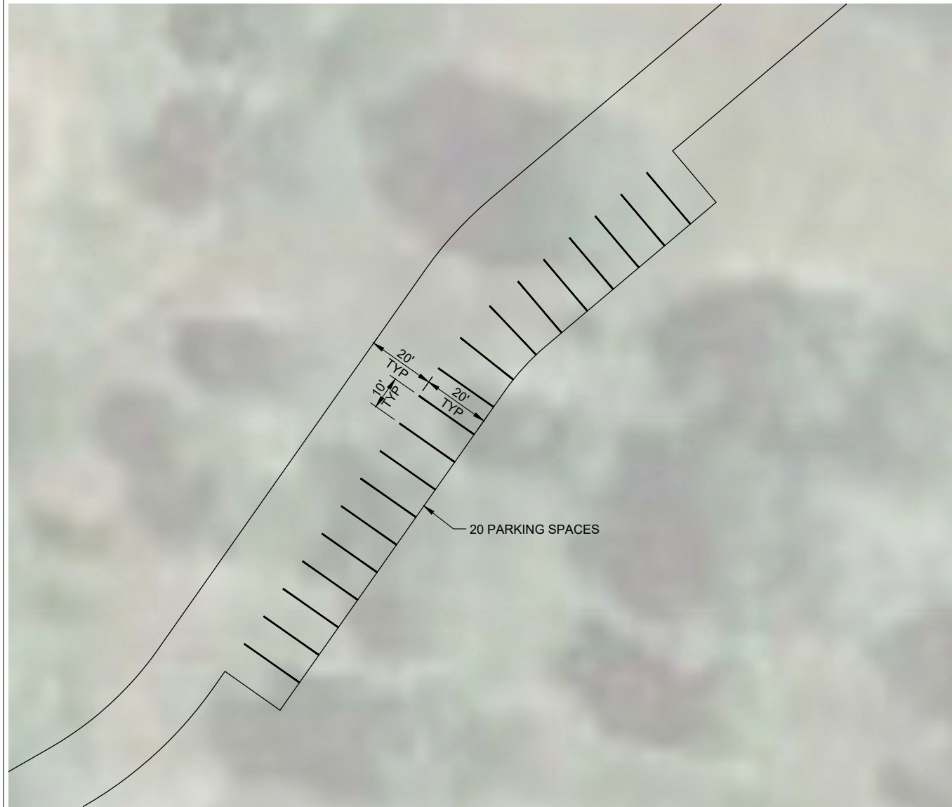
5 OVERFLOW PARKING AREA SCALE: 1" = 40' 0 20 40 80 U.S. SURVEY FEET
