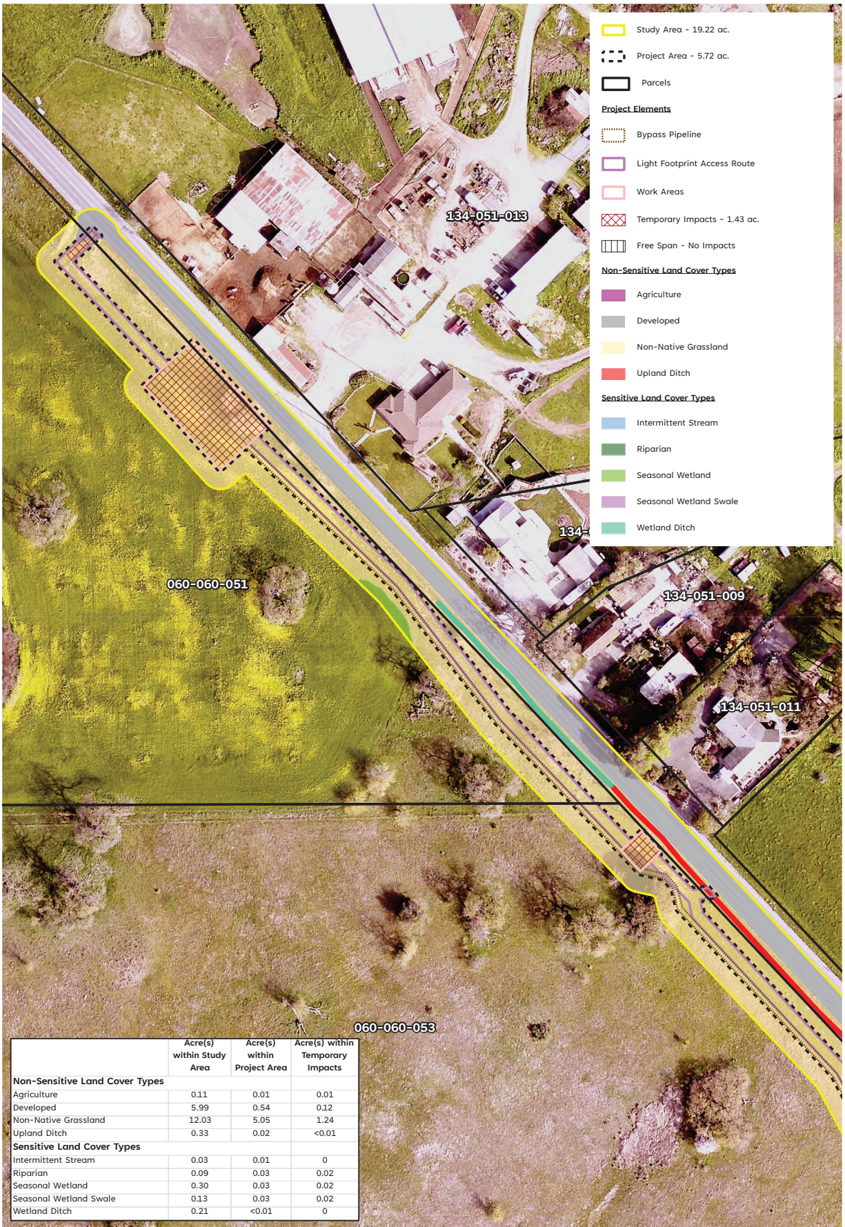
Figure 4-2. Project Design Plans and Impacts (Sheet 1)
