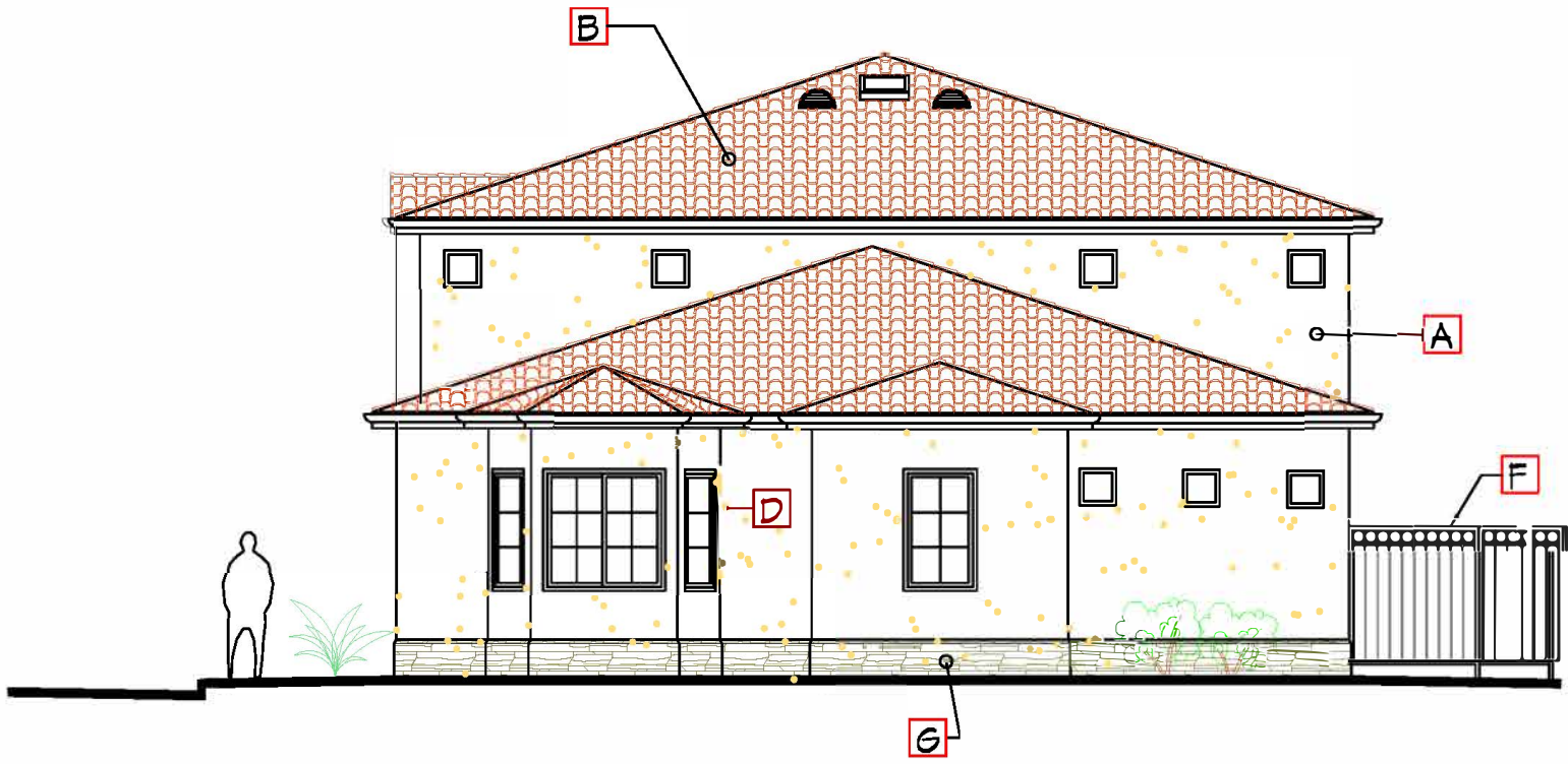
2 SOUTH ELEVATION BUILDING #1 (BUILDING #3 SIMILAR / #2 & #4 REVERSE) A-2.2 1/8"=1'-0"
