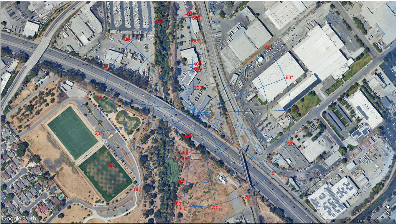
Figure 4. Site satellite photo overlay of distances and angles from proposed digital billboard site, corresponding to calculated illuminance figures in fc provided in Table 1.
