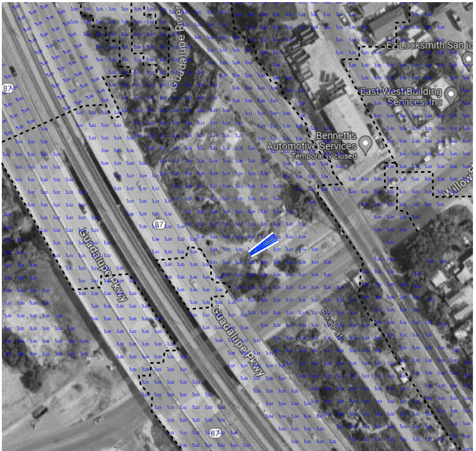
Photometry plan showing the lighting levels (in footcandles) on the ground and roadway surfaces. Points are spaced 30' apart for visibility.
