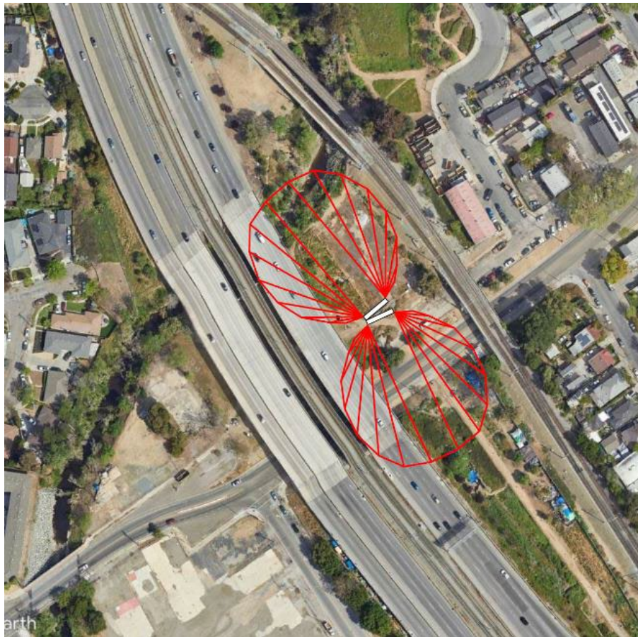
Image 3: Boundary of Night Illuminance of 0.3 Foot-Candles Using Focused Light Technology
