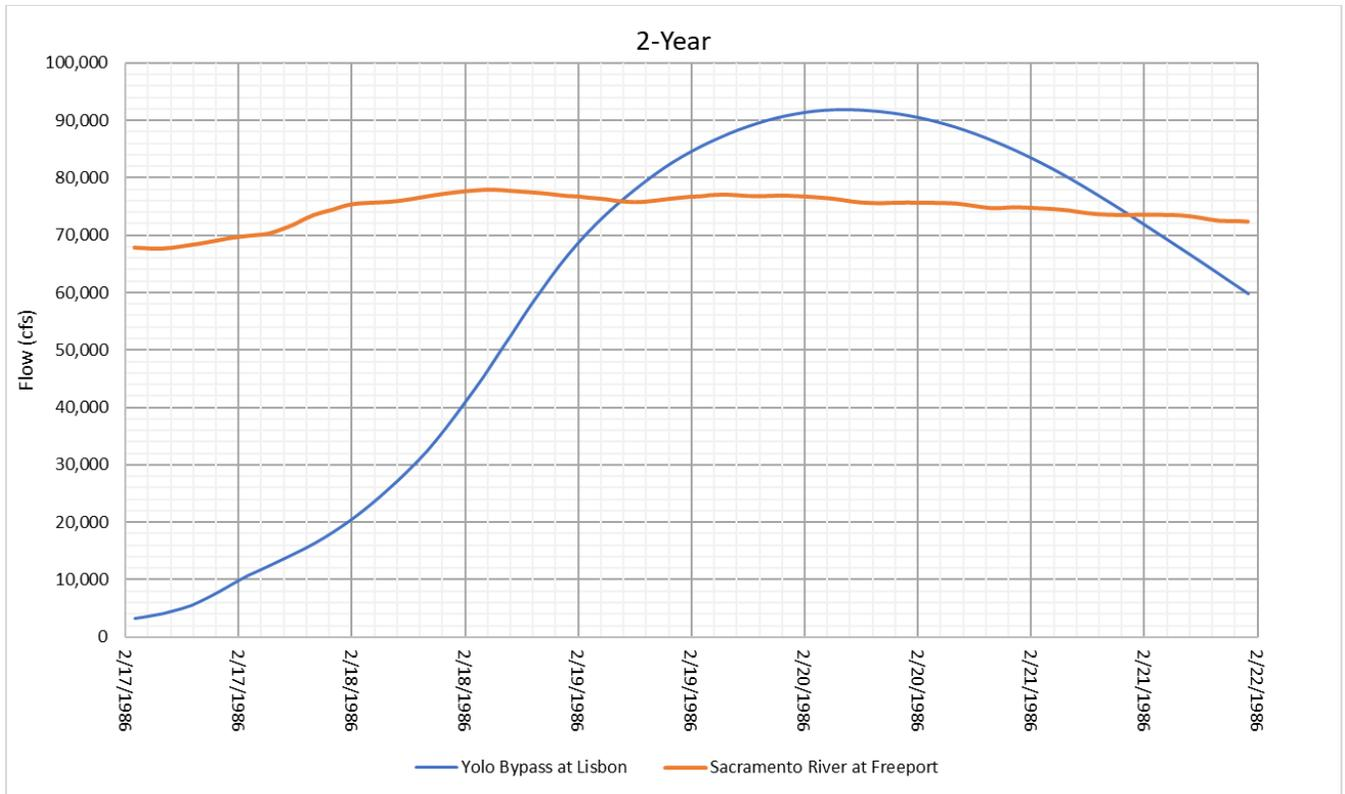
Figure 12. 2-Year Flow Hydrographs for Upstream Boundary Conditions
