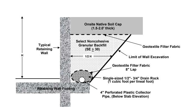
**Notes:** This system consists of a geotextile fabric-wrapped gravel envelope. Collection is with a 4-inch diameter perforated plastic pipe embedded in the gravel envelope and tied to a 4-inch diameter non-perforated plastic pipe which discharges at convenient locations. The outlet pipe should be placed such that the flow gradient is not less than 2.0 percent. The geotextile fabric-wrapped gravel envelope should be placed at a similar gradient
