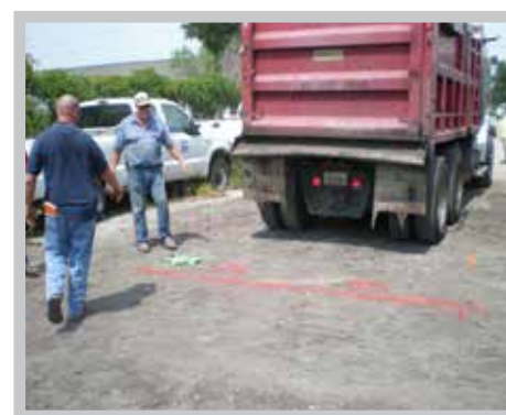
Truck (31 tons) backing over R-Tank.
