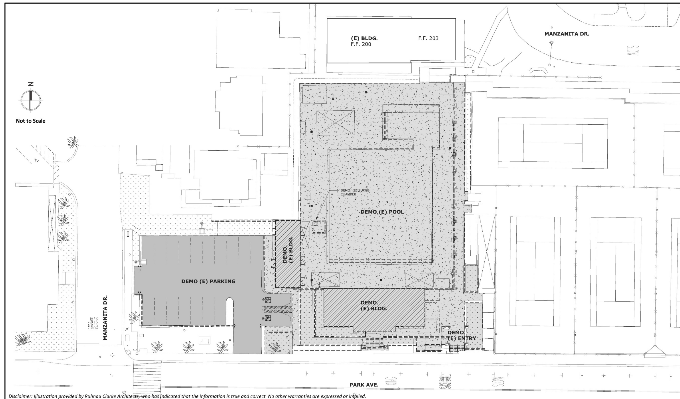
Figure 3.3-2 PROPOSED PROJECT DEMOLITION
