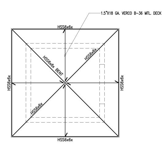
HIGH ROOF FRAMING PLAN
