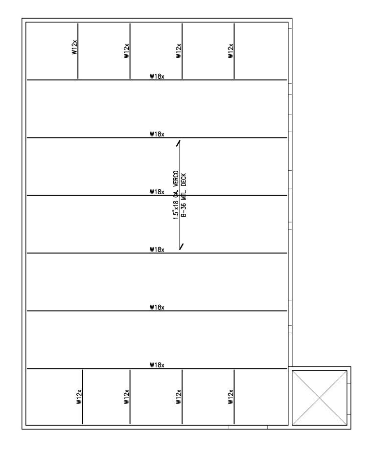
ROOF FRAMING PLAN SCALE:  $\frac{1}{8}$ " = 1'-0"
