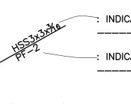
: INDICATES STEEL OR WOOD COLUMN SIZE. SEE DETAIL \_\_\_\_ FOR STEEL COLUMN BASE PLATE, U.N.O. : INDICATES CONCRETE FOOTING. SEE DETAIL \_\_\_\_ FOR ADDITIONAL INFORMATION.
