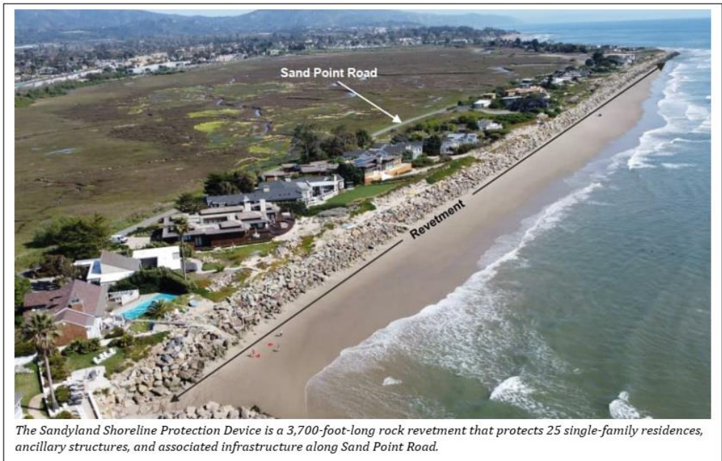
Figure 1. Figure showing the existing rock revetment wall in front of 25 homes below Carpinteria Marsh, Santa Barbara County.
