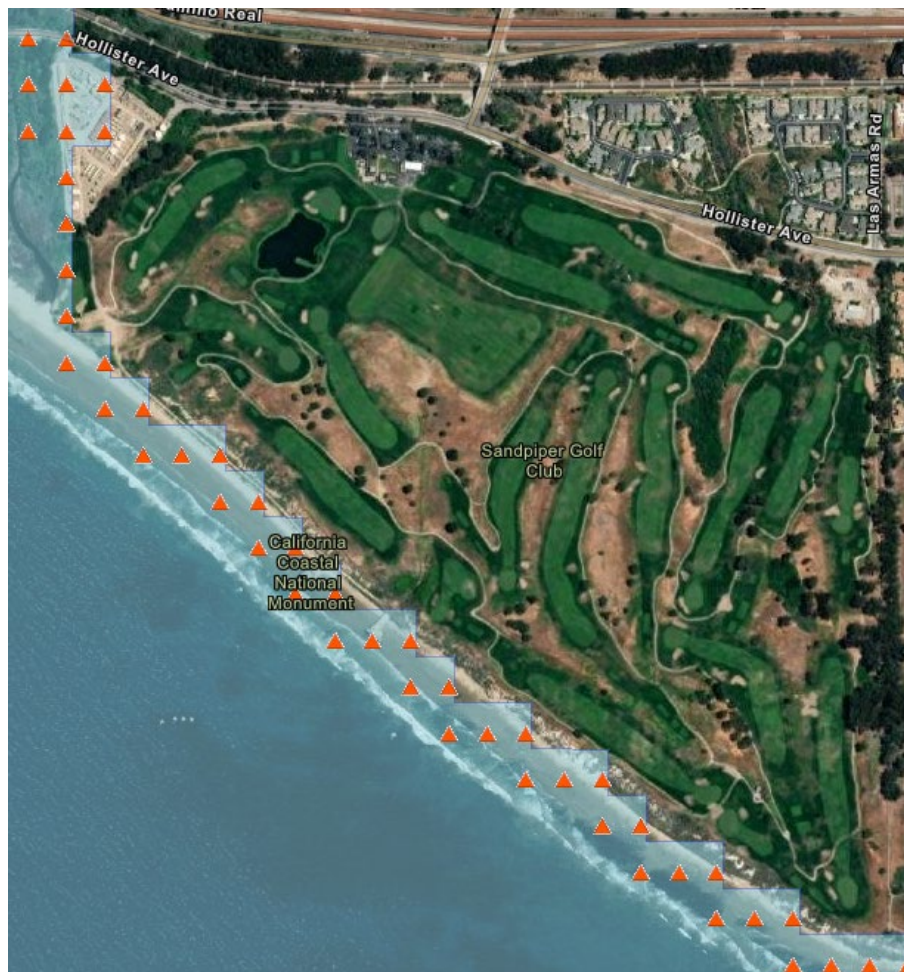
Figure 12. ASCE 7-16 Tsunami Hazard Tool displaying tsunami runup limits (blue shaded polygon and orange points)
