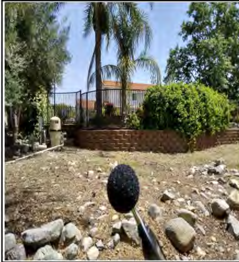
STNM2 looking W towards backyard of 5220 Mayberry Ave, Alta Loma. Pool water pump (left side of picture) is constantly on during 15 minute measurement.
