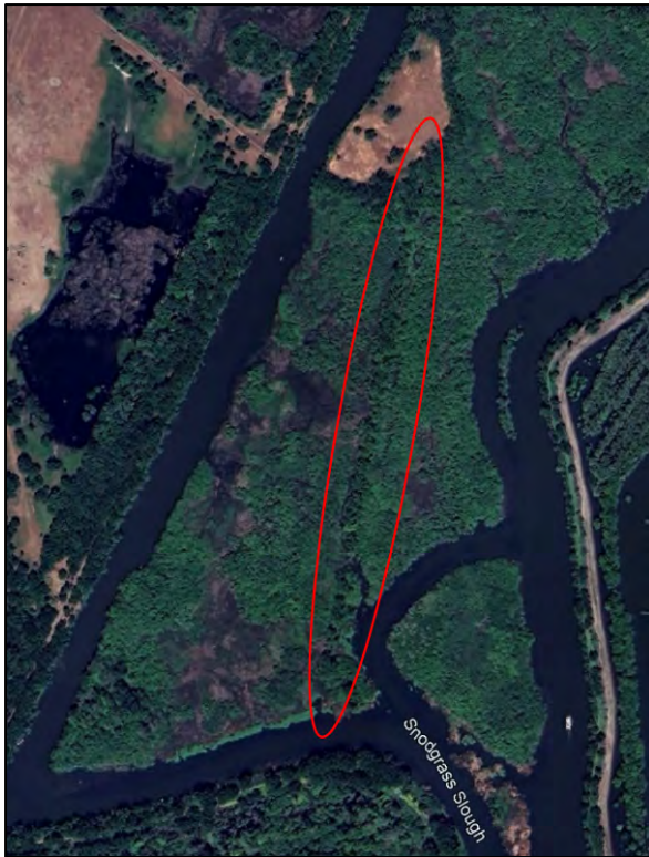
Photograph 6: Straight lines of trees growing on elevated mounds mark the locations of the SLS 877 levee (left) and SLS 764 levee (right); Google Earth imagery, May 12, 2023, annotated by JRP.
