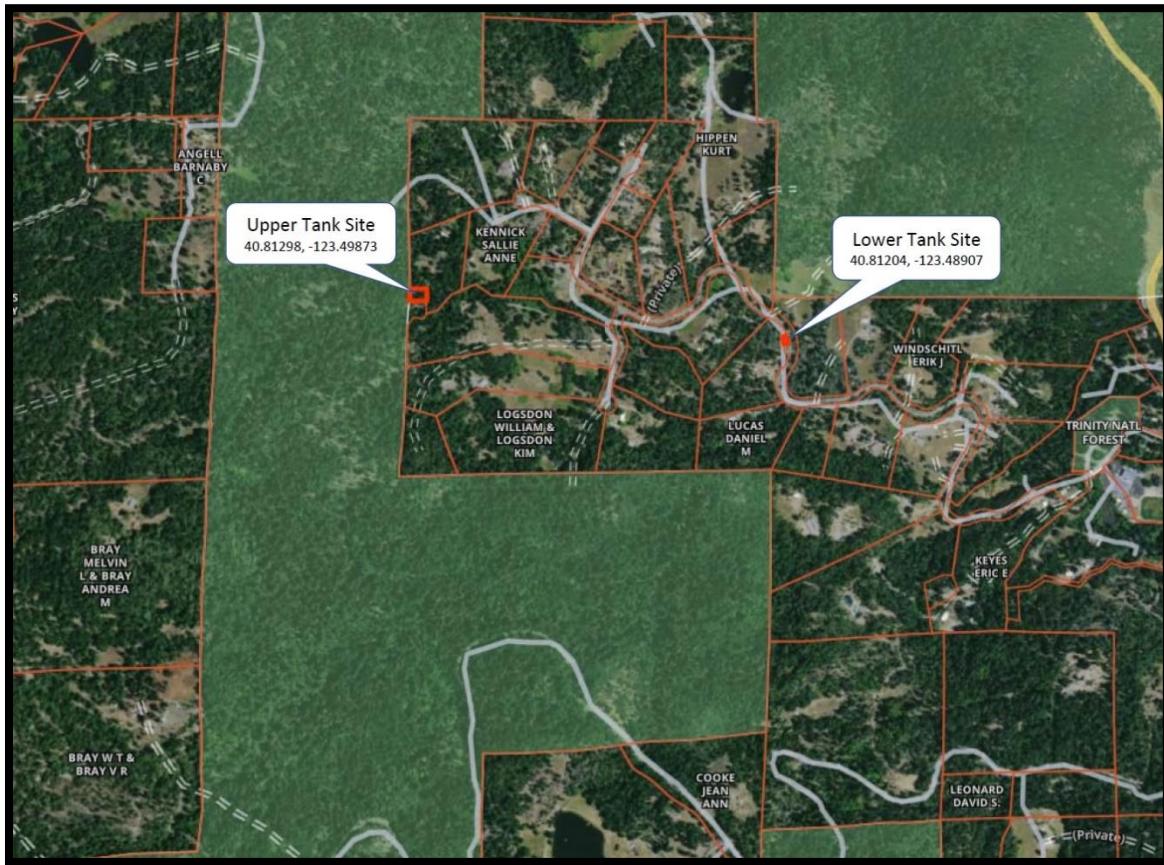
Figure 3. Project plan map, showing the locations proposed for water storage tank placement; courtesy of Trinity Valley Consulting Engineers, Willow Creek.
