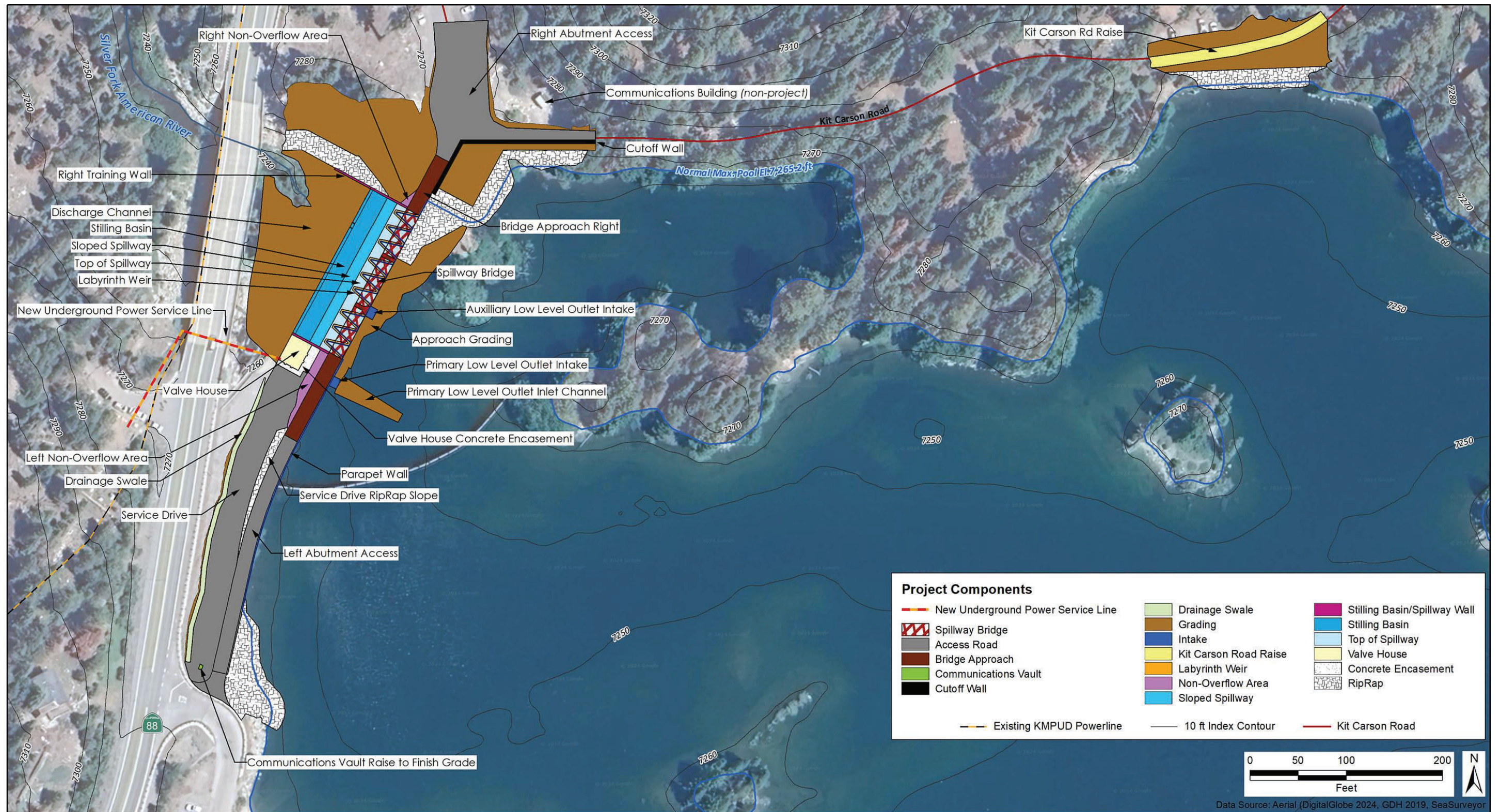
Figure 2. Proposed Replacement Dam, Spillway, and Appurtenances
